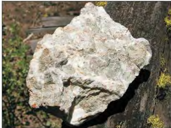
Figure 5. A 12-inch sample of silicified andesite breccia taken in the 400 level adit. Note pyritization in clasts and silica veinlets.
